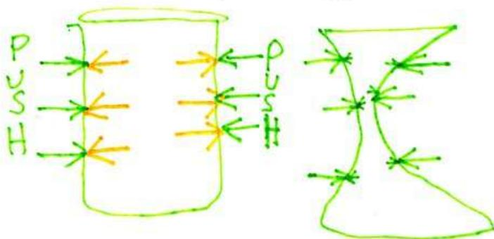
The can collapsed because suddenly the push from inside the can became very small.
