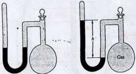
The difference h is the measure of the pressure of the gas inside the flask. If h is equal to 6.5 cm, calculate the pressure in the flask in the following units: 65 cm = 65 mm < millimeter
